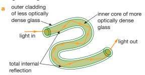
As the fibres are very narrow, light entering the inner core always strikes the boundary of the two glasses at an angle that is greater than the critical angle. This means that all the light is reflected (total internal reflection).
