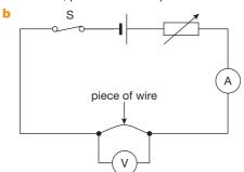
c Close the switch and record the readings on the ammeter and voltmeter. Use the variable resistor to change the resistance and take new readings. Repeat this at least six times. A graph of *I* against *V* should show a straight line passing through the origin, confirming Ohm's law.
