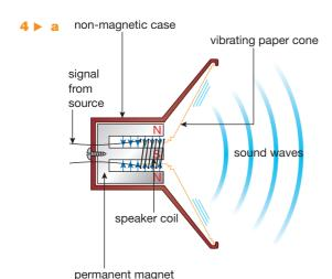
**b** Varying electric currents from the source create magnetic fields (around the speaker coil); the strength and direction of these fields change as the current changes. These changes make the speaker vibrate, creating the sound waves we hear.
