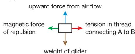
**ii** Newton's third law states that for every action there is an equal and opposite reaction. This means that glider A experiences an unbalanced magnetic force to the left from B and glider B experiences an unbalanced magnetic force to the right from A and that each of these forces is the same size. (3)
