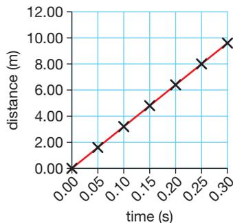
$$\begin{aligned} \text{gradient} &= \frac{\text{distance}}{\text{time}} \\ &= \frac{8 \text{ m}}{0.25 \text{ s}} \\ &= 32 \text{ m/s} \end{aligned}$$
