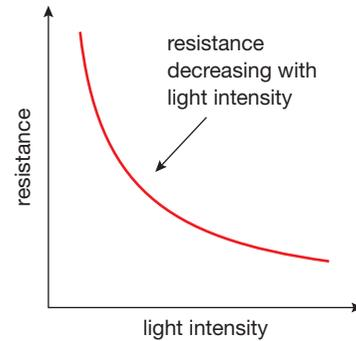
**b** Thermistors can be used in temperature circuits such as fire alarms and thermostats. LDRs can be used in light-sensitive circuits such as automatic lighting controls.
