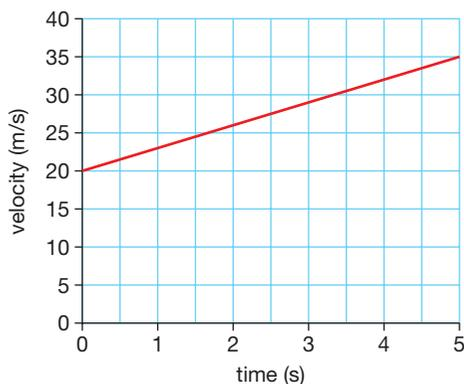
b Distance travelled is given by the area under the graph. (Divide area into a rectangle and a triangle.)
