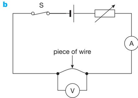
**c** Close the switch and take readings on ammeter and voltmeter. Alter the variable resistor and take new readings. Repeat this at least six times. A graph of  $I$  against  $V$  will show a straight line passing through the origin, confirming Ohm's law.
