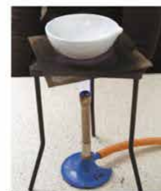
D | Hot equipment is a hazard when heating to dryness.
