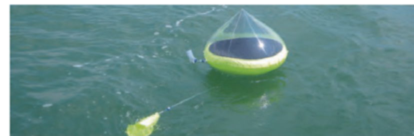
E | An inflatable solar still may be part of the emergency supplies on the life rafts of an ocean-going ship.
