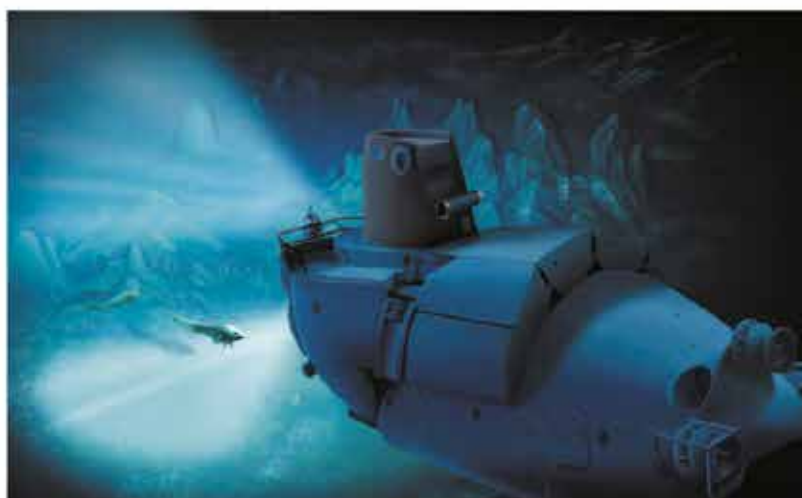
C | The submersible Alvin is used for scientific exploration of the sea bed. Its top speed is just over 3 km/h and it has a crew of two.
