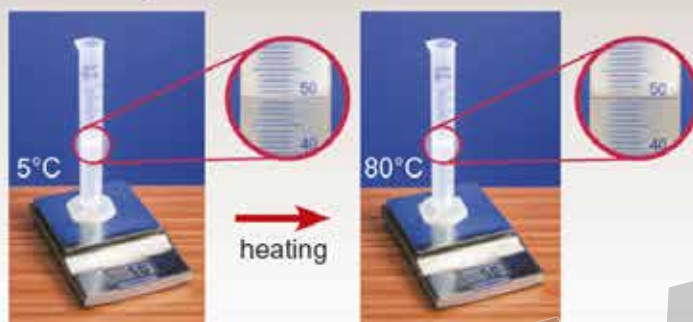
B | When the water is heated its mass does not change but its volume increases. This means that its density decreases.
