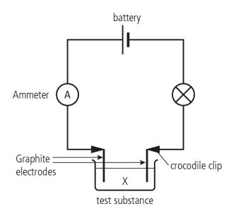
**B** Submerge the electrodes in the solution to be tested. If an analogue ammeter (galvanometer) is used, just record the deviation of the galvanometer needle instead. Record your observations in Table 2.
