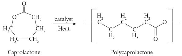
Polycaprolactone is easily sourced. It is sold as small white pellets for arts and crafts. Its thermal properties, exceptional mechanical and chemical properties, and its biocompatibility and biodegradability, have made it an ideal material for applications ranging from casual 3D printing to biomedical tissue engineering, and even for targeted drug delivery.
