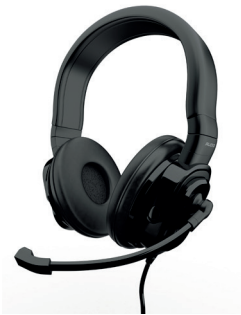
▲ Figure 1.48 This headset contains a microphone and headphone speakers
