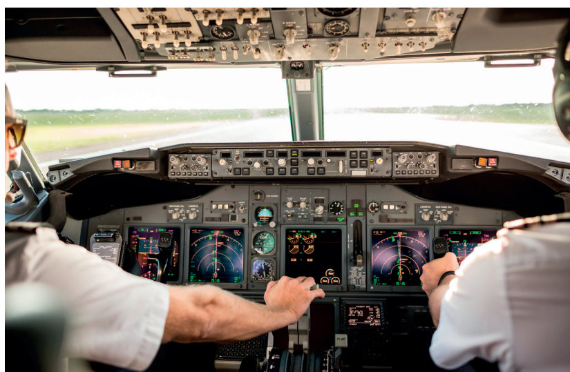
▲ Figure 1.60 Sensors are used in aircraft and data from them are displayed to the flight crew on instruments in the cockpit
