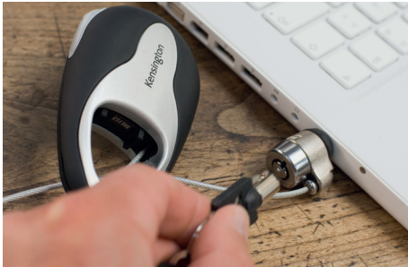
▲ Figure 1.33 A Kensington security lock in use
