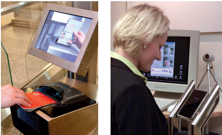
▲ Figure 1.55 Some passports now contain a chip that holds biometric data about the passport holder that is compared with the results of biometric scans carried out at airports
