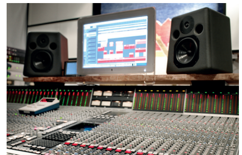
▲ Figure 1.69 A pair of speakers is required for stereo sound because one is used for the left side and one is used for the right side
