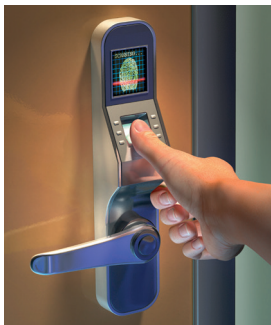
▲ Figure 1.51 A fingerprint scanner detects unique patterns in your fingerprints
