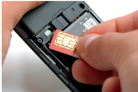
▲ Figure 1.7 The SIM card from a mobile phone
