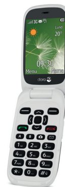
▲ Figure 1.9 Some mobile phones use tactile keypads, which are more responsive than other keypads, and give the user a choice of on-screen text size and colours
