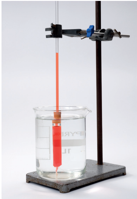
▲ Figure 2.3 Water enters the Visking tubing 'sausage' by osmosis. This causes the level of liquid in the capillary tube to rise. In the photograph, the contents of the Visking tubing have had a red dye added to them to make it easier to see the movement of the liquid.
