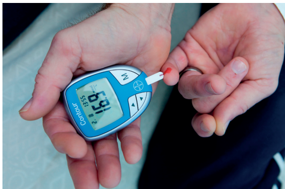
▲ Figure 3.15 A biosensor for measuring blood glucose levels. A drop of blood has been placed onto the probe of the biosensor.
