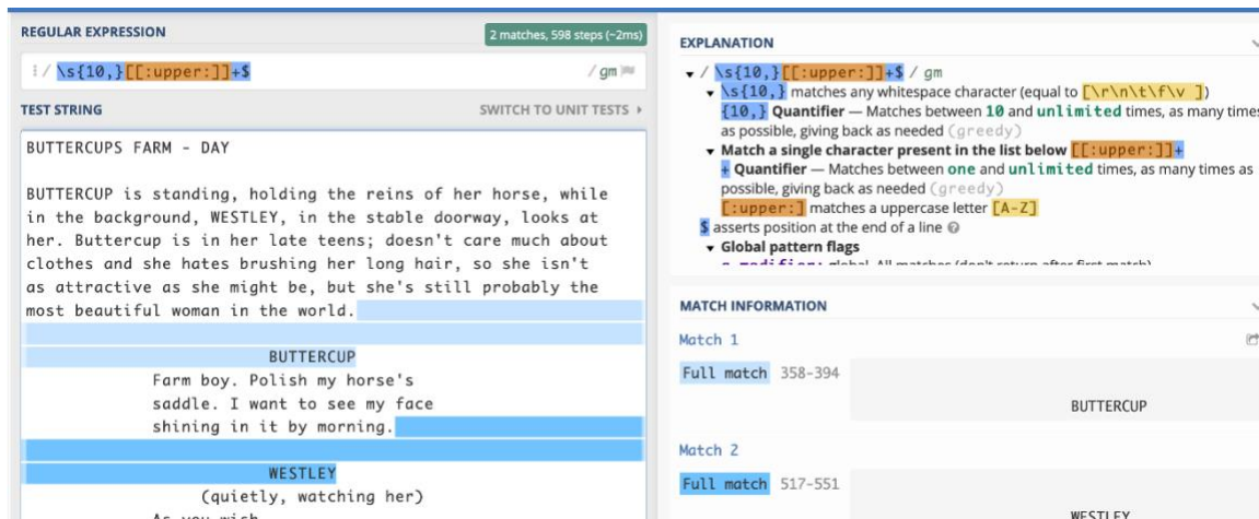
Figure 3. Screen shot of regular expression testing using RegEx 101. ( https://regex101.com ). This regular expression identifies characters (in shades of blue) with speaking roles from the movie script for The Princess Bride (downloaded from the Internet Movie Script Database, https://www.imsdb.com/ ). The top right of the web page includes an explanation for the regular expression.
