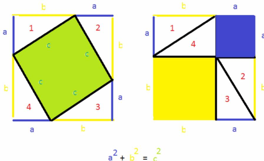
In the left-side figure, we have four equivalent triangles with legs of lengths  $a$  and  $b$  stacked in a way that gives us a giant square with sides of length  $a + b$ . This placement also gives a center
