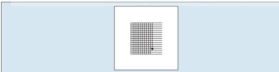
Assume the size of the lattice is **16** by **16** and the distance between two lines in the lattice is **10** pixels (lines 6–21). The program first draws the lattice in gray color. It sets the color to gray (line 7), uses the **for** loop (lines 9–13) to draw the horizontal lines, and the **for** loop (lines 17–21) to draw the vertical lines.
