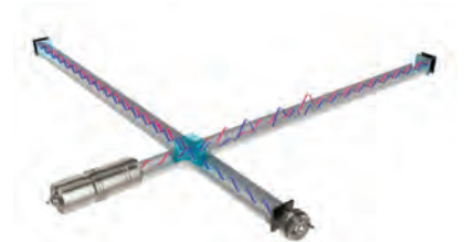
FIGURE 7.11.4 Gravitational wave detection: perpendicular ultra-high vacuum tubes are used to detect gravitational waves. Gravitational waves will cause extremely small changes in the lasers (red and blue lines) moving through the tubes which can be detected.
