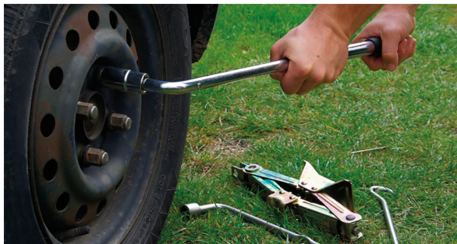
FIGURE 2.1.8 Loosening the wheel nuts with an extended handle spanner will increase the torque on the nut.
