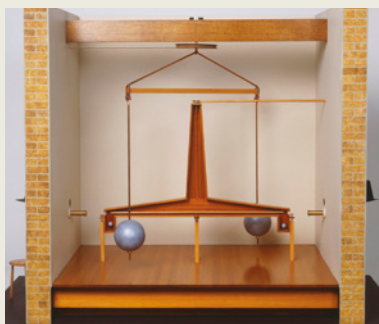
FIGURE 1.1.3 Henry Cavendish used a torsion balance to measure the small twisting force created by the gravitational attraction of lead balls. A very similar method is still in use in introductory labs in senior secondary schools and universities today.
