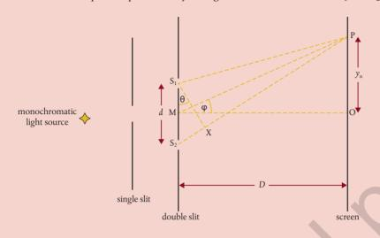
The diagram below (not drawn to scale) shows an arrangement for observing the interference pattern produced by the light from two narrow slits  $S_1$  and  $S_2$ .
