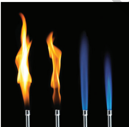
FIGURE 2.5.2 The yellow flame of a Bunsen burner is due to incomplete combustion and produces carbon as a product. The blue flame is a hotter flame that occurs when the air hole is open and more oxygen is allowed to react, resulting in complete combustion.
