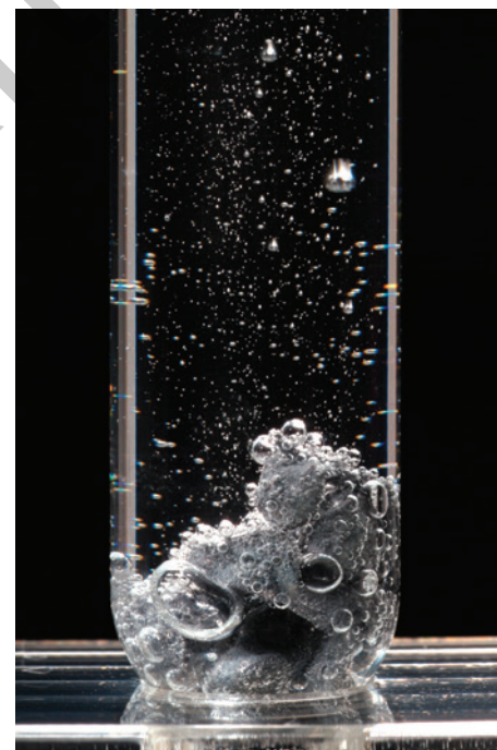
FIGURE 2.1.3 When zinc comes into contact with hydrochloric acid, it reacts almost immediately. The reactants have sufficient energy to 'overcome' the activation energy barrier.
