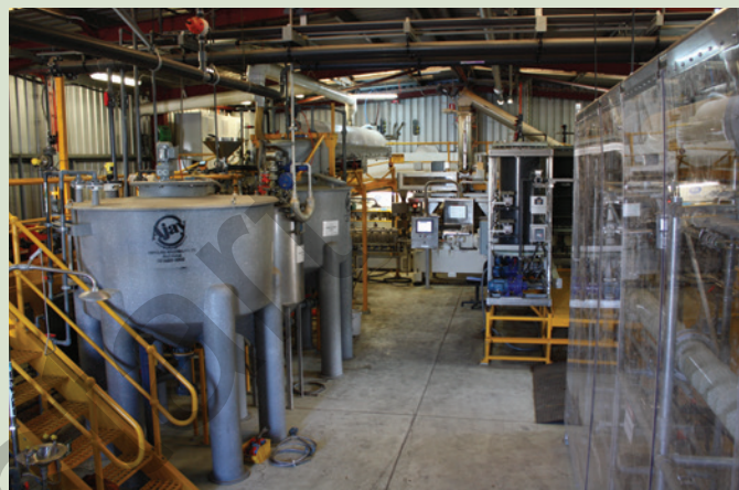
FIGURE 2.4.8 Ethtec trial plant with biomass fermentation tanks on the left of the photo
