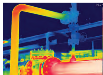
FIGURE 3.9.8 A thermal camera uses infrared light to investigate the temperature of machinery as it operates; by analysing this data the efficiency and safety of the machinery can be evaluated
