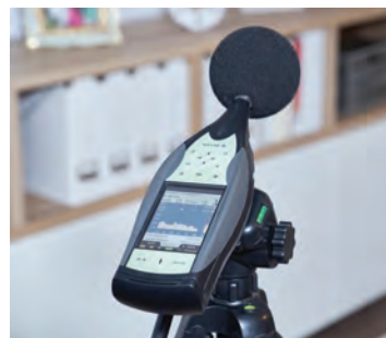
FIGURE 3.6.9 Sound level meter measuring the level of noise in a house
