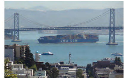
FIGURE 2.6.6 This cargo ship is passing under the bridge at low tide to ensure there is enough clearance.
