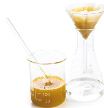
FIGURE 2.3.2 Filtration of muddy water. Solid mud and clay particles suspended in water can be separated from the liquid water by the process of filtration.
