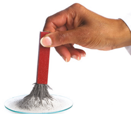
FIGURE 2.3.6 A magnet is used to separate iron filings from the non-magnetic sand particles.
