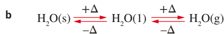
FIGURE 2.1.3 (a) Processes describing the changes of state between solids, liquids and gases. (b) The melting, boiling, condensing and freezing of water can be represented using chemical formulas and chemical equations. The bracketed letters, (s), (l) and (g), represent the solid, liquid and gaseous states of water. The '+ \Delta ' and '- \Delta ' symbols refer to the need to 'add heat' or 'subtract heat' to induce the changes of state indicated.
