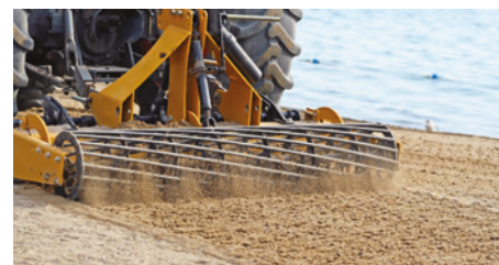
FIGURE 2.3.1 Queensland beaches are cleaned by tractors dragging a rotating mesh drum to sieve large objects such as rocks, shells and other rubbish.
