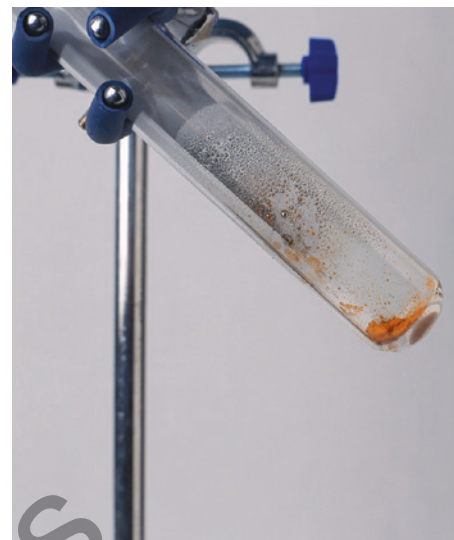
FIGURE 2.1.7 The red powder in this test-tube is mercury(II) oxide ( \text{HgO} ). If you look closely at the test-tube, you will see beads of liquid mercury forming from the decomposition of the compound.
