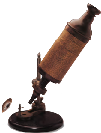
FIGURE 1.3.2 Robert Hooke's microscope
