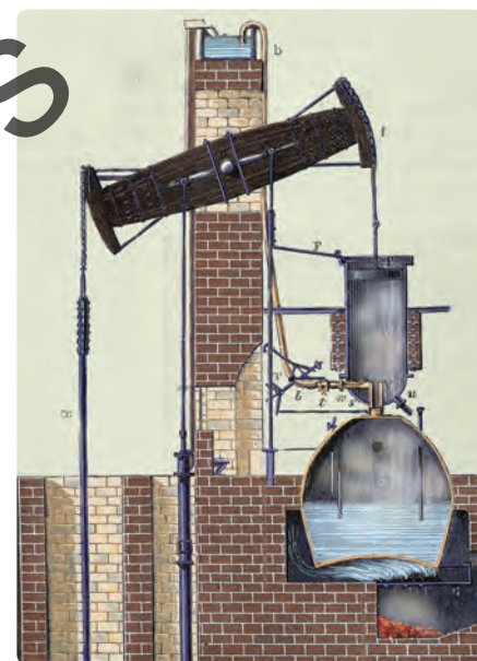
Source 2.2.2 The atmospheric steam engine, invented by Thomas Newcomen in 1712
