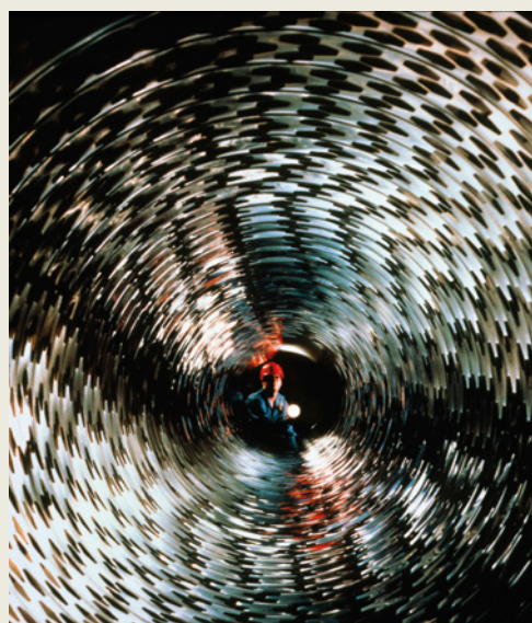
FIGURE 1.3.9 The interior view of a gas centrifuge used for enriching uranium for nuclear power stations
