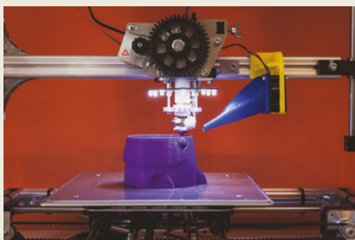
FIGURE 1.1.3 This 3D printer uses an acrylonitrile–butadiene–styrene polymer to make an object.
