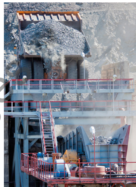
FIGURE 1.3.1 After ore is mined, it is placed into a hopper crusher like this one. The ore is then pulverised. The smallest pieces fall through a sieve, while the larger pieces are crushed further.
