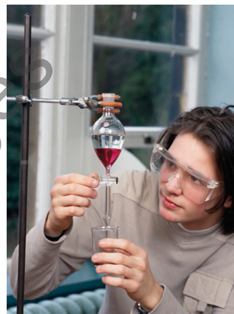
FIGURE 1.3.6 Separation funnels are often used in organic chemistry where many organic solvents display significantly different densities from aqueous solutions.
