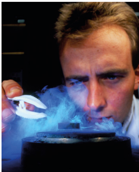
FIGURE 1.1.4 A small cylindrical magnet being levitated above a liquid nitrogen-cooled, superconducting ceramic by the Meissner effect
