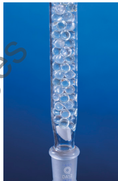
FIGURE 1.3.11 A glass fractionating column filled with glass beads
