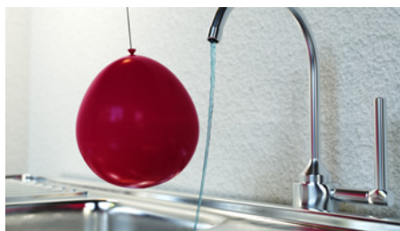
FIGURE 3.3.1 A stream of water bending near a statically charged balloon
