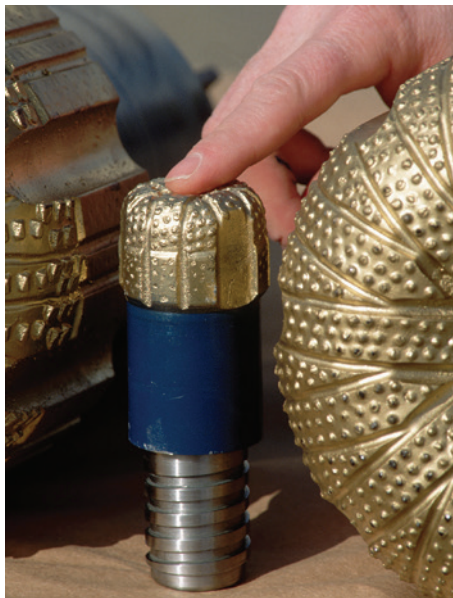
FIGURE 3.5.5 Diamond-tipped drills used to drill through rock in the oil mining industry
