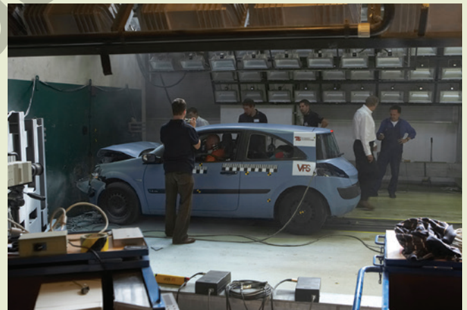
FIGURE 3.2.7 The Australian New Car Assessment Program (ANCAP) assesses the crashworthiness of new cars. This car has just crashed at 50 \text{ km h}^{-1} into a 5 \text{ t} concrete block. The crumpling effect can clearly be seen.
