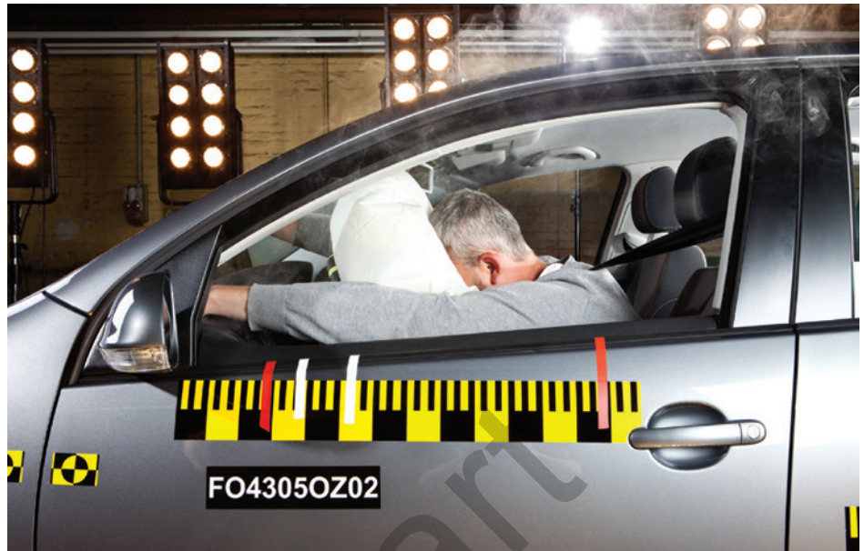
FIGURE 3.2.4 Airbags reduce the force on passengers by extending the time it takes for them to stop in the event of a collision.
