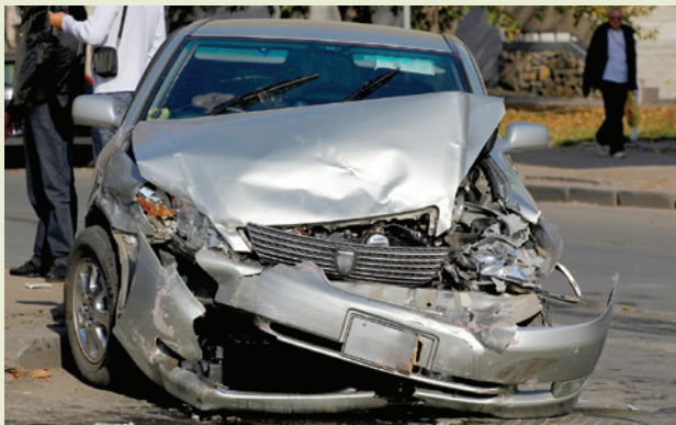
FIGURE 3.2.6 Cars are designed with weak points in their chassis that enable the car to crumple in the event of a collision. This extends the time over which the cars come to rest and so reduces the size of the forces acting on the occupants.
