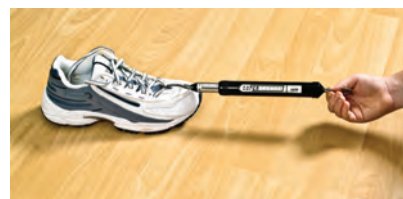
FIGURE 1.6.1 A newton meter can be used to measure how much force is required to slide this shoe across the ground.
