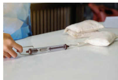
FIGURE 8 Force being measured with a newton meter
