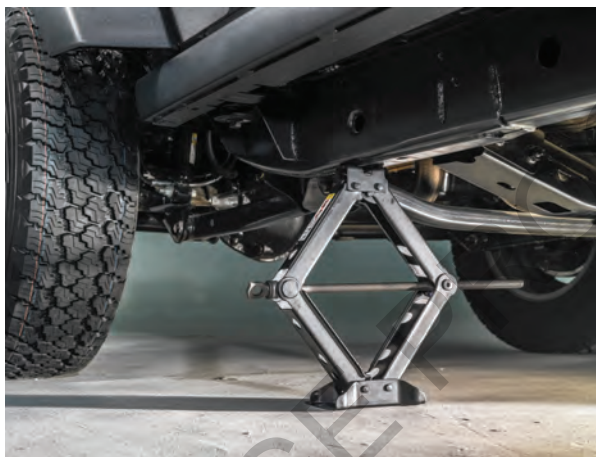
FIGURE 1.13.12 A small rotational force on a car jack can apply a strong upward force on the car, lifting it off the ground.
