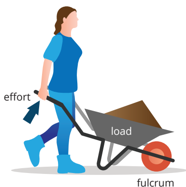
FIGURE 1.9.4 Wheelbarrows are a common example of second-class levers used to lift heavy loads.
