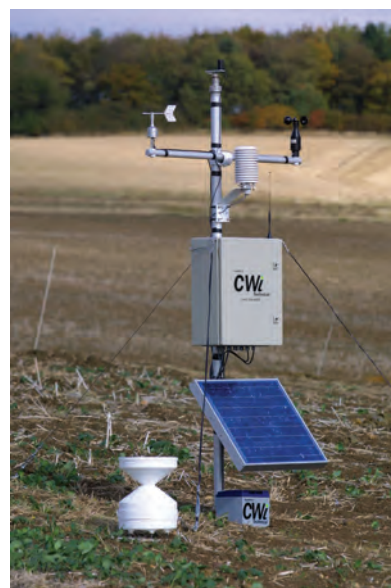
FIGURE 3 A weather station is a useful tool for determining rainfall and solar radiation (sunlight).
