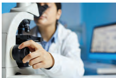
FIGURE 1.13.13 The focus knobs on a microscope convert large movements of the knob into much finer movements of the lens.
