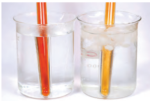
FIGURE 2.3.6 Equilibrium mixtures of \text{NO}_2 and \text{N}_2\text{O}_4 in hot water and ice. Heating the mixture favours the formation of brown \text{NO}_2 gas.
