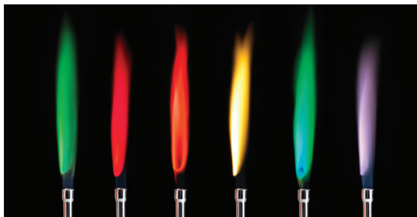
FIGURE 2.2.2 The colour of the flame is determined by the different metal compounds present and can be used to identify these metals. The flame colours shown here are for (from left to right): barium (yellow-green), lithium (crimson), strontium (scarlet), sodium (yellow), copper (green) and potassium (lilac).
