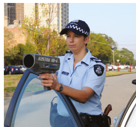
FIGURE 1.2.2 To avoid a systematic error, make sure that you are using measuring equipment correctly. Laser speed guns, for example, need to be placed on a stationary support so the aim point is held on a single target point for the duration of the read.
