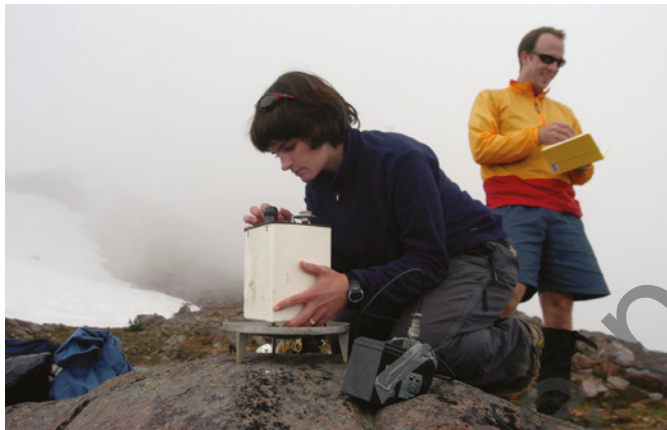
FIGURE 5.2.6 A gravimeter can be used to measure the strength of the local gravitational field.
