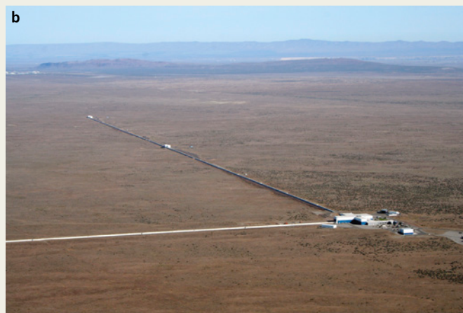
FIGURE 5.2.12 (a) Monash University (Australia) astrophysicist Chris Whittle in the optics vacuum chamber at LIGO, Washington USA, assisting with the replacement of an interferometer mirror. The cleanroom suit minimises dust, which can foul the equipment. (b) LIGO's observatory in Washington state, USA, showing the two perpendicular arms of the facility.
