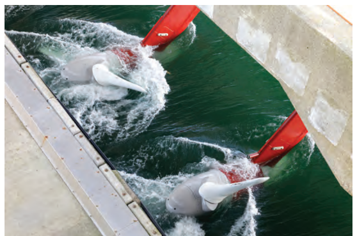
FIGURE 2.6.10 Tidal currents can turn turbines which are used to generate electricity.
