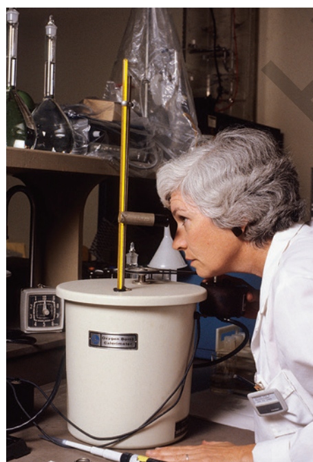
FIGURE 3.3.7 Bomb calorimeter temperature changes being observed by a laboratory technician
